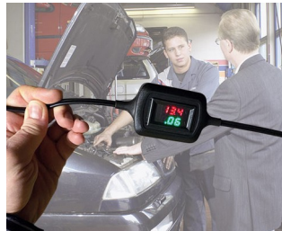
Voltage and current display during trickle charging
