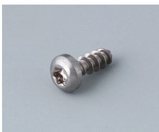
A0308132 Self-tapping screw 0.118" x 0.315" (T10) Stainless steel
