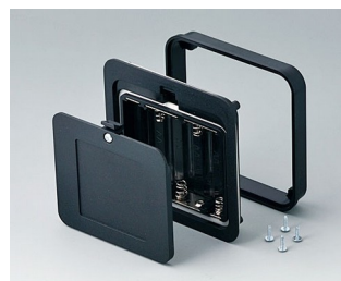
A9338119 Battery compartment kit, 5 x AA ABS (UL 94 HB) black RAL 9005 3.66"x3.86" IP 54
