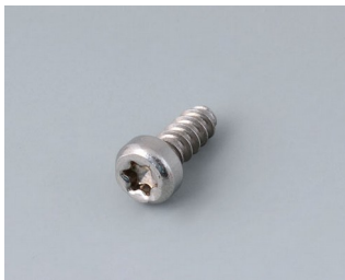
A0325060 Self-tapping screw 0.098" x 0.236" (T8) Stainless steel
