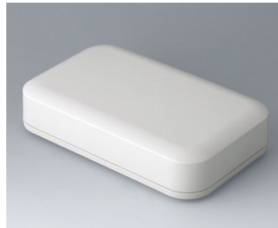
A9461107 EVOTEC 200, Vers. I ASA+PC (UL 94 V-0) off-white RAL 9002 7.87"x4.88"x1.77" IP 65 opt., IP 40
