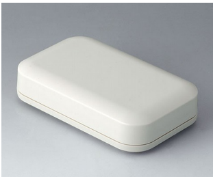
A9431107 EVOTEC 125, Vers. I ASA+PC (UL 94 V-0) off-white RAL 9002 4.92"x3.07"x1.18" IP 65 opt., IP 40
