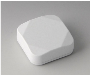
B1802117 MINI-DATA-BOX S40, flat ASA+PC (UL 94 V-0) traffic white RAL 9016 1.57"x1.57"x0.59" IP 65 opt., IP 40
