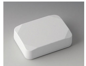
B1824217 MINI-DATA-BOX E50, high ASA+PC (UL 94 V-0) traffic white RAL 9016 2.76"x1.97"x0.79" IP 65 opt., IP 40
