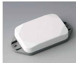
B1822126 MINI-DATA-BOX EF40, flat, with flanges ASA+PC (UL 94 V-0) traffic white RAL 9016 2.36"x1.57"x0.59" IP 65 opt., IP 40
