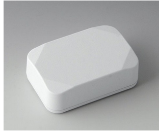
B1822217 MINI-DATA-BOX E40, high ASA+PC (UL 94 V-0) traffic white RAL 9016 2.36"x1.57"x0.79" IP 65 opt., IP 40
