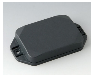
B1824128 MINI-DATA-BOX EF50, flat, with flanges ASA+PC (UL 94 V-0) anthracite gray RAL 7016 2.76"x1.97"x0.59" IP 65 opt., IP 40
