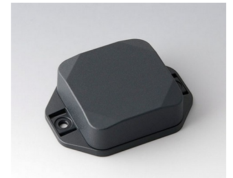
B1804228 MINI-DATA-BOX SF50, high, with flanges ASA+PC (UL 94 V-0) anthracite gray RAL 7016 1.97"x1.97"x0.79" IP 65 opt., IP 40
