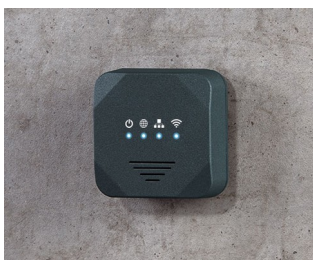
Wireless Access Point
