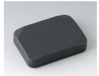
B1824118 MINI-DATA-BOX E50, flat ASA+PC (UL 94 V-0) anthracite gray RAL 7016 2.76"x1.97"x0.59" IP 65 opt., IP 40
