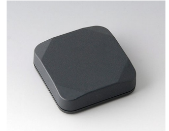
B1804118 MINI-DATA-BOX S50, flat ASA+PC (UL 94 V-0) anthracite gray RAL 7016 1.97"x1.97"x0.59" IP 65 opt., IP 40
