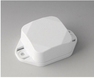
B1802227 MINI-DATA-BOX SF40, high, with flanges ASA+PC (UL 94 V-0) traffic white RAL 9016 1.57"x1.57"x0.79" IP 65 opt., IP 40
