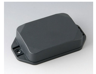
B1824228 MINI-DATA-BOX EF50, high, with flanges ASA+PC (UL 94 V-0) anthracite gray RAL 7016 2.76"x1.97"x0.79" IP 65 opt., IP 40
