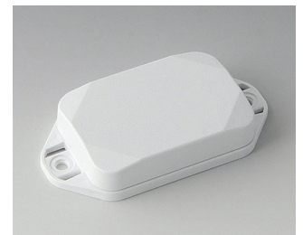
B1822127 MINI-DATA-BOX EF40, flat, with flanges ASA+PC (UL 94 V-0) traffic white RAL 9016 2.36"x1.57"x0.59" IP 65 opt., IP 40
