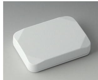
B1824117 MINI-DATA-BOX E50, flat ASA+PC (UL 94 V-0) traffic white RAL 9016 2.76"x1.97"x0.59" IP 65 opt., IP 40
