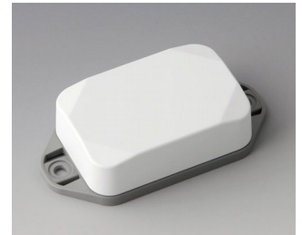
B1822226 MINI-DATA-BOX EF40, high, with flanges ASA+PC (UL 94 V-0) traffic white RAL 9016 2.36"x1.57"x0.79" IP 65 opt., IP 40
