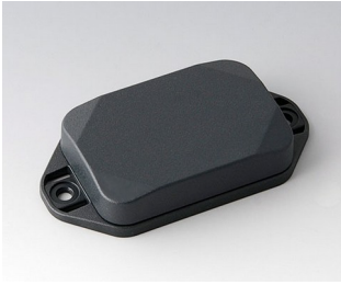
B1822128 MINI-DATA-BOX EF40, flat, with flanges ASA+PC (UL 94 V-0) anthracite gray RAL 7016 2.36"x1.57"x0.59" IP 65 opt., IP 40
