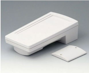
A9046107 HAND-TERMINAL M, Vers. I PC+ABS (UL 94 V-0) off-white RAL 9002 8.66"x4.72"x2.56" IP 65 opt.
