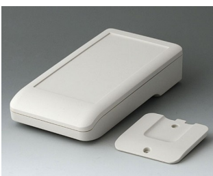
A9006207 DATEC-COMPACT M ASA+PC (UL 94 V-0) off-white RAL 9002 6.77"x3.62"x1.54" IP 65
