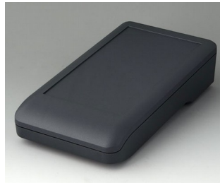
A9007108 DATEC-COMPACT L ASA+PC (UL 94 V-0) lava 8.11"x4.33"x1.85" IP 65
