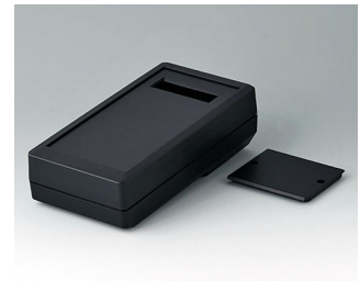
A9074229 DATEC-MOBIL-BOX M, Vers. II, high ABS (UL 94 HB) black RAL 9005 7.68"x3.98"x2.32" IP 65 opt.
