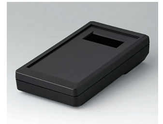
A9073219 DATEC-MOBIL-BOX S, Vers. II ABS (UL 94 HB) black RAL 9005 5.98"x3.27"x1.32" IP 65 opt.
