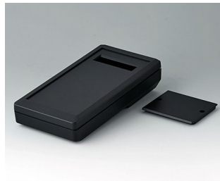
A9074309 DATEC-MOBIL-BOX M, Vers. III ABS (UL 94 HB) black RAL 9005 7.68"x3.98"x1.73" IP 65 opt.
