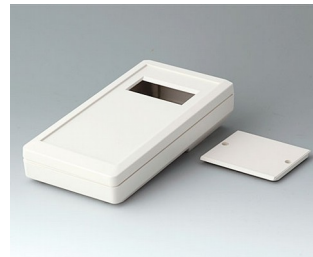
A9074407 DATEC-MOBIL-BOX M, Vers. IV ABS (UL 94 HB) off-white RAL 9002 7.68"x3.98"x1.73" IP 65 opt.
