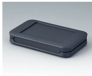
A9050108 SOFT-CASE S ABS (UL 94 HB) lava 2.01"x3.23"x0.55" IP 54 opt., IP 40
