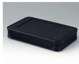
A9053209 SOFT-CASE XL PMMA (IR) (UL 94 HB) black RAL 9005 3.62"x5.91"x1.10" IP 40
