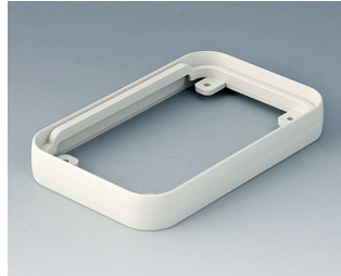
A9150017 Intermediate ring S ABS (UL 94 HB) off-white RAL 9002 2.13"x3.35"x0.47"
