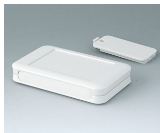
A9051117 SOFT-CASE M ABS (UL 94 HB) off-white RAL 9002 2.56"x4.13"x0.75" IP 40
