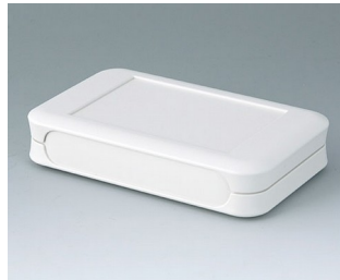
A9052107 SOFT-CASE L ABS (UL 94 HB) off-white RAL 9002 2.87"x4.61"x0.94" IP 54 opt., IP 40
