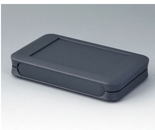
A9051108 SOFT-CASE M ABS (UL 94 HB) lava 2.56"x4.13"x0.75" IP 54 opt., IP 40
