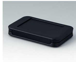
A9050209 SOFT-CASE S PMMA (IR) (UL 94 HB) black RAL 9005 2.01"x3.23"x0.55" IP 54 opt., IP 40
