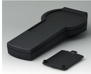
A9076109 DATEC-CONTROL XS, Vers. I ABS (UL 94 HB) black RAL 9005 7.87"x3.70"x1.56" IP 65 opt.
