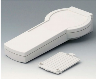
A9076107 DATEC-CONTROL XS, Vers. I ABS (UL 94 HB) off-white RAL 9002 7.87"x3.70"x1.56" IP 65 opt.
