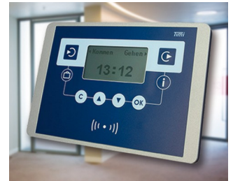
Terminal for personnel time recording
