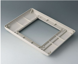
B4046707 Bottom part L flat, version I ABS (UL 94 HB) off-white RAL 9002 10.83"x7.68"x1.04" IP 54 opt.
