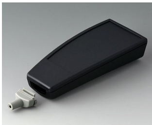
A9067139 SMART-CASE L, Vers. IV ABS (UL 94 HB) black RAL 9005 5.51"x2.47"x1.20" IP 65 opt., IP 40
