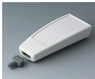
A9067147 SMART-CASE L, Vers. V ABS (UL 94 HB) off-white RAL 9002 5.51"x2.47"x1.20" IP 65 opt., IP 40
