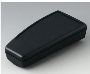
A9066419 SMART-CASE M, Vers. VI PMMA (IR) (UL 94 HB) black RAL 9005 3.78"x1.85"x0.94" IP 40
