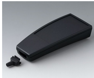
A9068339 SMART-CASE XL, Vers. IV ABS (UL 94 HB) black RAL 9005 6.61"x2.93"x1.39" IP 65 opt., IP 40
