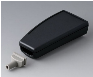
A9066129 SMART-CASE M, Vers. III ABS (UL 94 HB) black RAL 9005 3.78"x1.85"x0.94" IP 40
