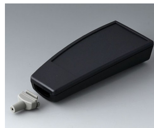
A9067149 SMART-CASE L, Vers. V ABS (UL 94 HB) black RAL 9005 5.51"x2.47"x1.20" IP 65 opt., IP 40
