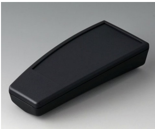
A9067219 SMART-CASE L, Vers. II PMMA (IR) (UL 94 HB) black RAL 9005 5.51"x2.47"x1.20" IP 65 opt., IP 40
