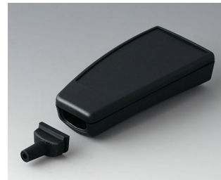
A9066339 SMART-CASE M, Vers. IV ABS (UL 94 HB) black RAL 9005 3.78"x1.85"x0.94" IP 40
