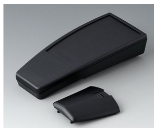
A9068109 SMART-CASE XL, Vers. I ABS (UL 94 HB) black RAL 9005 6.61"x2.93"x1.39" IP 40
