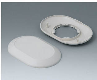
B5015007 Bottom and top part O160 F ABS (UL 94 HB) off-white RAL 9002 6.30"x4.33"x1.18"
