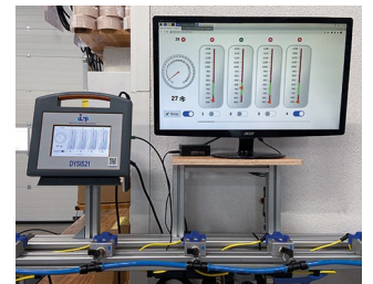
Monitoring system for cleaning nozzles
