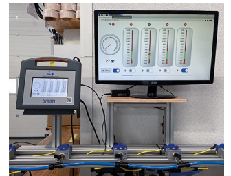
Monitoring system for cleaning nozzles
