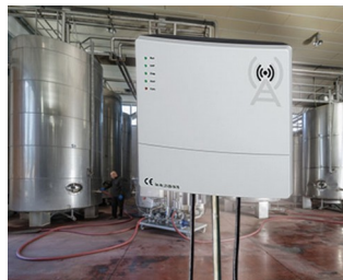
Gateway for the automation of production plants
