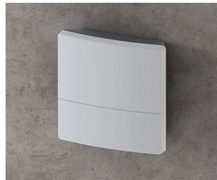
B3214201 NET-BOX 140, Vers. II ASA+PC (UL 94 V-0) light gray RAL 7035 5.51"x5.51"x1.83" IP 65 opt.
