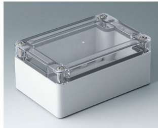
C7012014 IN-BOX ABS/PC (UL 94 HB) light gray RAL 7035 4.80"x3.23"x2.17" IP 66, IP 67, IK 07
