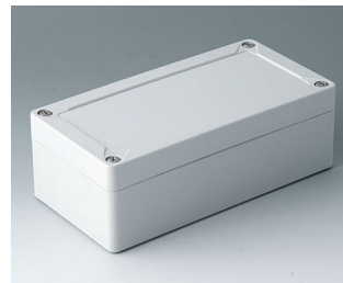
C7016012 IN-BOX PC light gray RAL 7035 6.38"x3.23"x2.17" IP 66, IP 67, IK 08
