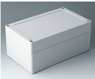
C7020061 IN-BOX ABS (UL 94 HB) light gray RAL 7035 7.95"x4.80"x3.54" IP 66, IP 67, IK 07
