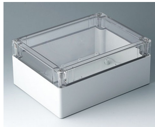
C7021074 IN-BOX ABS/PC (UL 94 HB) light gray RAL 7035 7.95"x5.98"x3.54" IP 66, IP 67, IK 07
