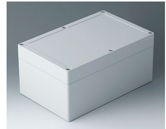
C7025091 IN-BOX ABS (UL 94 HB) light gray RAL 7035 9.92"x6.38"x4.72" IP 66, IP 67, IK 07
