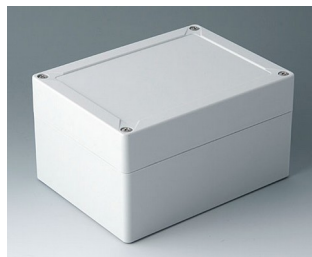
C7016062 IN-BOX PC light gray RAL 7035 6.38"x4.80"x3.54" IP 66, IP 67, IK 08
