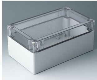
C7020064 IN-BOX ABS/PC (UL 94 HB) light gray RAL 7035 7.95"x4.80"x3.54" IP 66, IP 67, IK 07
