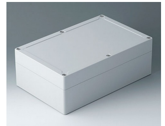
C7025081 IN-BOX ABS (UL 94 HB) light gray RAL 7035 9.92"x6.38"x3.54" IP 66, IP 67, IK 07
