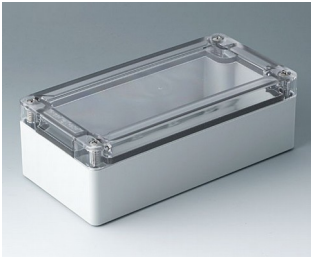
C7016015 IN-BOX PC light gray RAL 7035 6.38"x3.23"x2.17" IP 66, IP 67, IK 08
