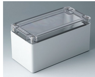
C7016024 IN-BOX ABS/PC (UL 94 HB) light gray RAL 7035 6.38"x3.23"x3.35" IP 66, IP 67, IK 07
