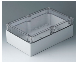
C7025084 IN-BOX ABS/PC (UL 94 HB) light gray RAL 7035 9.92"x6.38"x3.54" IP 66, IP 67, IK 07
