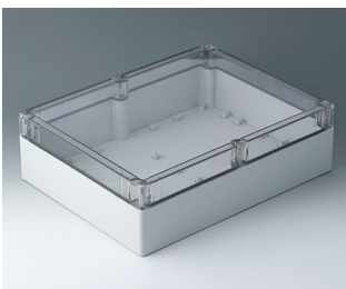
C7030104 IN-BOX ABS/PC (UL 94 HB) light gray RAL 7035 11.89"x9.13"x3.54" IP 66, IP 67, IK 07
