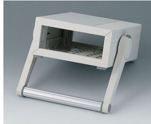
B2213107 MEDITEC E 160, with handle bar ABS (UL 94 HB) off-white RAL 9002 6.30"x7.87"x2.91" IP 40
