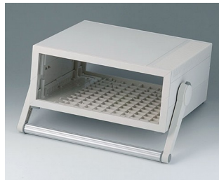
B2210307 MEDITEC D 220, with handle bar ABS (UL 94 HB) off-white RAL 9002 11.42"x10.24"x4.88" IP 40
