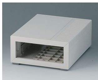
B2213007 MEDITEC E 160, without handle bar ABS (UL 94 HB) off-white RAL 9002 6.30"x7.87"x2.91" IP 40
