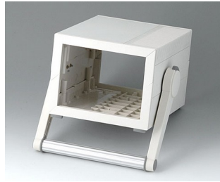
B2213307 MEDITEC E 160, with handle bar ABS (UL 94 HB) off-white RAL 9002 6.30"x7.87"x4.88" IP 40
