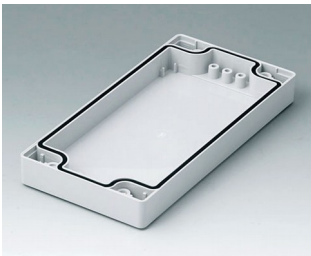
C0081601 Case shell 3.150", with groove ABS (UL 94 HB) light gray RAL 7035 6.30"x3.15"x0.79"
