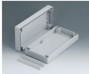
C2012242 ROBUST-BOX WIDTH 4.724", Vers. II PC (UL 94 HB) light gray RAL 7035 9.45"x4.72"x2.36" IP 66
