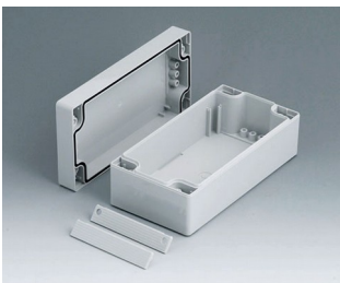
C2008161 ROBUST-BOX WIDTH 3.150", Vers. I ABS (UL 94 HB) light gray RAL 7035 6.30"x3.15"x2.36" IP 66
