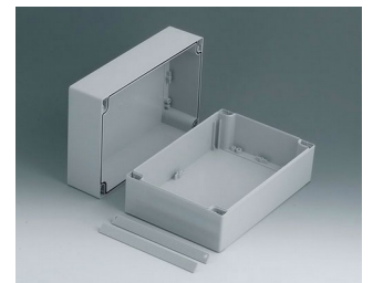
C2416242 ROBUST-BOX WIDTH 6.299", Vers. II PC (UL 94 HB) light gray RAL 7035 9.45"x6.30"x4.72" IP 66
