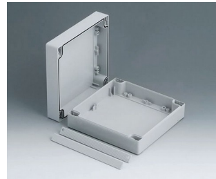
C2016161 ROBUST-BOX WIDTH 6.299", Vers. I ABS (UL 94 HB) light gray RAL 7035 6.30"x6.30"x2.36" IP 66
