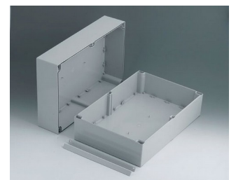
C2524361 ROBUST-BOX WIDTH 9.449", Vers. I ABS (UL 94 HB) light gray RAL 7035 14.17"x9.45"x6.30" IP 66
