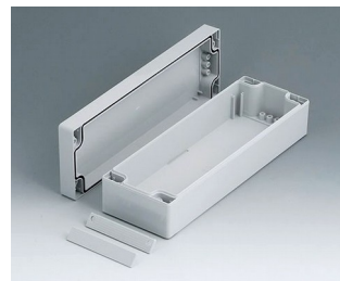
C2008241 ROBUST-BOX WIDTH 3.150", Vers. I ABS (UL 94 HB) light gray RAL 7035 9.45"x3.15"x2.36" IP 66
