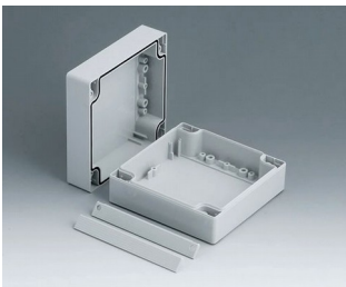
C2012121 ROBUST-BOX WIDTH 4.724", Vers. I ABS (UL 94 HB) light gray RAL 7035 4.72"x4.72"x2.36" IP 66
