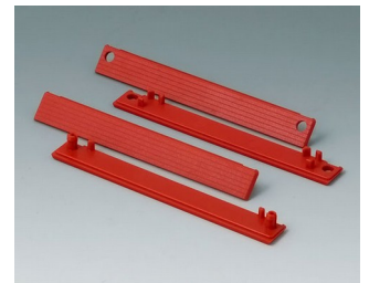
C2203124 Cover strips 4.724" PC (UL 94 HB) red RAL 3020
