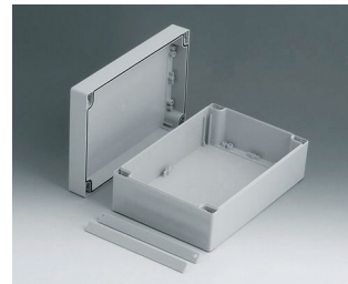
C2116241 ROBUST-BOX WIDTH 6.299", Vers. I ABS (UL 94 HB) light gray RAL 7035 9.45"x6.30"x3.54" IP 66
