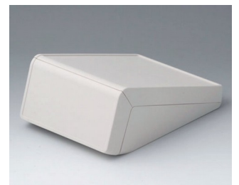
B4056137 UNITEC M, 0.02/0.06 ABS (UL 94 HB) off-white RAL 9002 5.83"x8.27"x3.15" IP 40
