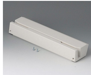
B4030917 Lid L with card slot, one piece ABS (UL 94 HB) off-white RAL 9002 10.55"x2.64"x1.50"
