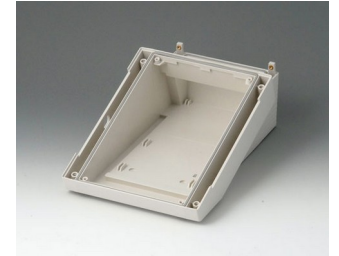
B4016317 DATEC-TERMINAL M, Vers. III ABS (UL 94 HB) off-white RAL 9002 6.61"x10.71"x3.98" IP 54 opt.
