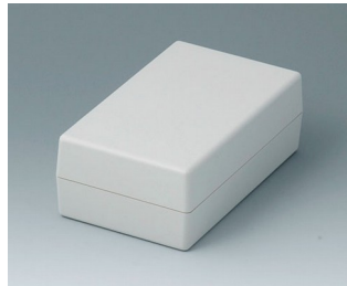
A9408441 SHELL-TYPE CASES G 155, Vers. I ABS (UL 94 HB) off-white RAL 9002 3.74"x6.22"x2.24" IP 65 opt.
