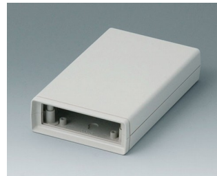
A9408333 SHELL-TYPE CASES V 155, Vers. I ABS (UL 94 HB) off-white RAL 9002 3.74"x6.22"x1.30"
