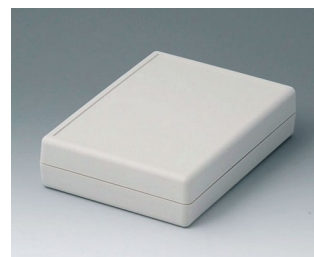
A9413351 SHELL-TYPE CASES G 190, Vers. I ABS (UL 94 HB) off-white RAL 9002 5.43"x7.48"x1.79" IP 65 opt.
