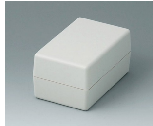
A9406441 SHELL-TYPE CASES G 110, Vers. I ABS (UL 94 HB) off-white RAL 9002 2.83"x4.49"x2.24" IP 65 opt.
