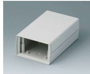
A9408443 SHELL-TYPE CASES V 155, Vers. I ABS (UL 94 HB) off-white RAL 9002 3.74"x6.22"x2.24"
