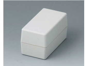
A9404441 SHELL-TYPE CASES G 85, Vers. I ABS (UL 94 HB) off-white RAL 9002 1.77"x3.35"x1.77" IP 65 opt.
