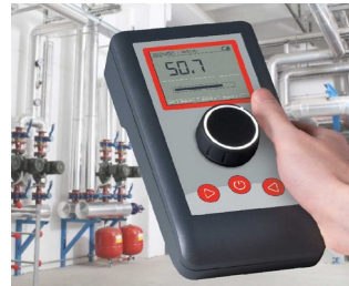
Find compressed air leaks using ultrasound
