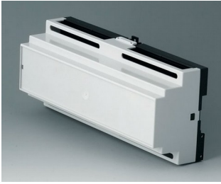
B6506111 RAILTEC B, 12 modules, Vers. I PC (UL 94 V-0) light gray RAL 7035 8.27"x3.54"x2.28"
