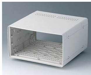
A0234170 EURO CASE 42 TE, without handle ABS (UL 94 HB) off-white RAL 9002 10.24"x9.84"x5.63"
