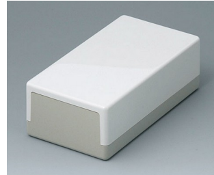
A9020065 FLAT-PACK CASES 120 N, Vers. I ABS (UL 94 HB) off-white RAL 9002 4.72"x2.56"x1.57" IP 40
