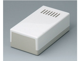
A9020265 FLAT-PACK CASE 120 S ABS (UL 94 HB) off-white RAL 9002 4.72"x2.56"x1.57"
