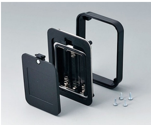
A9336119 Battery compartment kit, 3 x AA ABS (UL 94 HB) black RAL 9005 3.66"x2.72" IP 54
