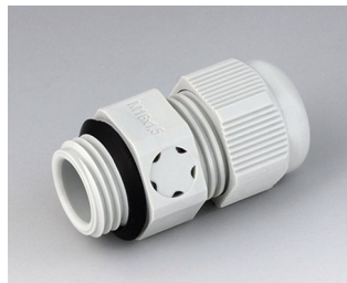
C2316917 Cable gland M16x0.059", pressure compensation PA light gray RAL 7035
