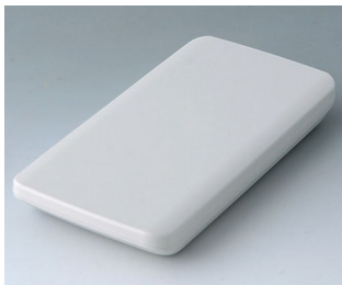
B5403107 SLIM-CASE M, Vers. I ASA+PC (UL 94 V-0) off-white RAL 9002 5.83"x2.91"x0.75" IP 65 opt., IP 40
