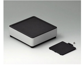
ES103059 SYNERGY S100 Aluminum AlMgSi 0.5 matt anodized 3.94"x3.94"x1.57" IP 40
