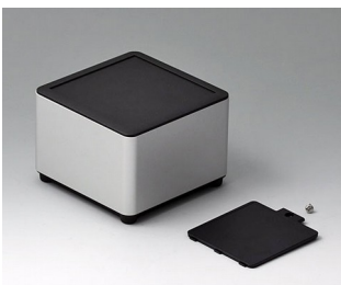
ES106059 SYNERGY S100 Aluminum AlMgSi 0.5 matt anodized 3.94"x3.94"x2.76" IP 40
