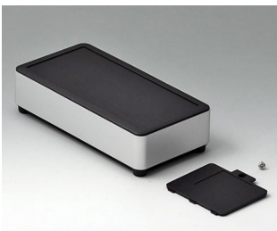
EE163059 SYNERGY E160 Aluminum AlMgSi 0.5 matt anodized 6.30"x3.15"x1.57" IP 40
