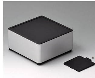
ES146059 SYNERGY S140 Aluminum AlMgSi 0.5 matt anodized 5.51"x5.51"x2.76" IP 40
