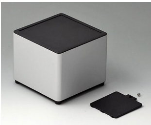
ES129059 SYNERGY S120 Aluminum AlMgSi 0.5 matt anodized 4.72"x4.72"x3.94" IP 40
