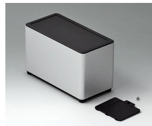
EE169059 SYNERGY E160 Aluminum AlMgSi 0.5 matt anodized 6.30"x3.15"x3.94" IP 40
