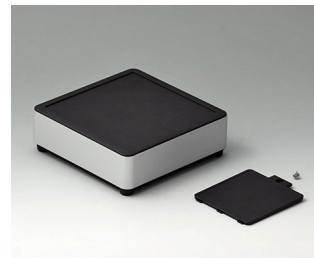
ES123059 SYNERGY S120 Aluminum AlMgSi 0.5 matt anodized 4.72"x4.72"x1.57" IP 40
