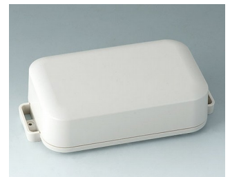
C3208207 EASYTEC 150 ASA+PC (UL 94 V-0) off-white RAL 9002 6.77"x3.66"x1.81" IP 65 opt., IP 40
