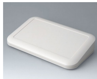
A9486107 EVOTEC 250, Vers. III ASA+PC (UL 94 V-0) off-white RAL 9002 9.84"x6.10"x2.13" IP 65 opt., IP 40
