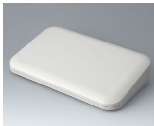
A9485107 EVOTEC 250, Vers. II ASA+PC (UL 94 V-0) off-white RAL 9002 9.84"x6.10"x2.13" IP 65 opt., IP 40
