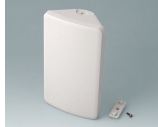
B4610107 SMART-CONTROL M, Vers. I ASA+PC (UL 94 V-0) off-white RAL 9002 6.81"x3.98"x2.32" IP 55 opt., IP 40
