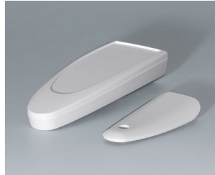
B2802017 STYLE-CASE S ASA (UL 94 HB) traffic white RAL 9016 4.84"x1.89"x0.94" IP 40
