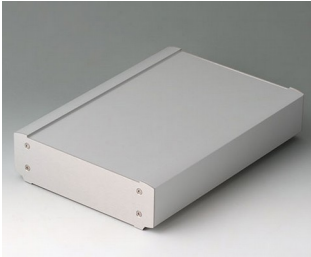
B3407033 SMART-TERMINAL 240 Aluminum AlMgSi 0.5 matt anodized 9.61"x6.69"x1.97"
