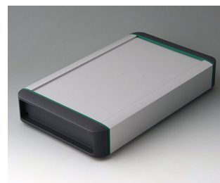
B3407031 SMART-TERMINAL 240 Aluminum AlMgSi 0.5 matt anodized 11.10"x6.69"x1.97" IP 54
